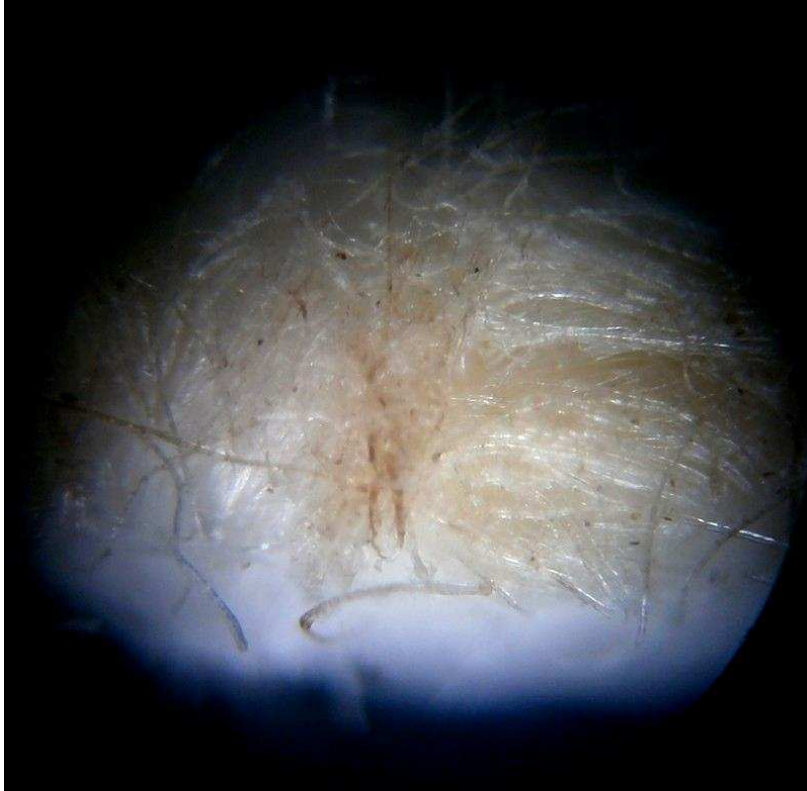
Fig.8: Very light Scorch. Highly colored portions of some superficial fibers
