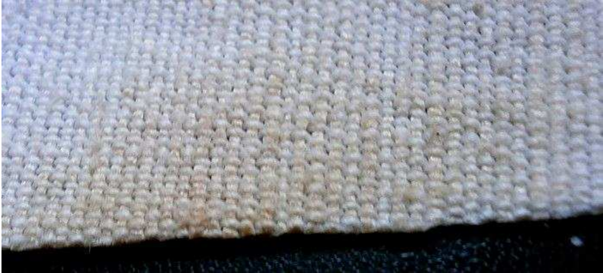
Fig. 15: cut in a lightly scorched area. The entire thickness of the colored threads is colored.
