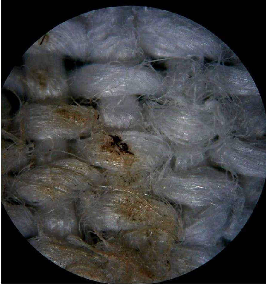
Fig.14: Light Scorch. Burnt fibers.
