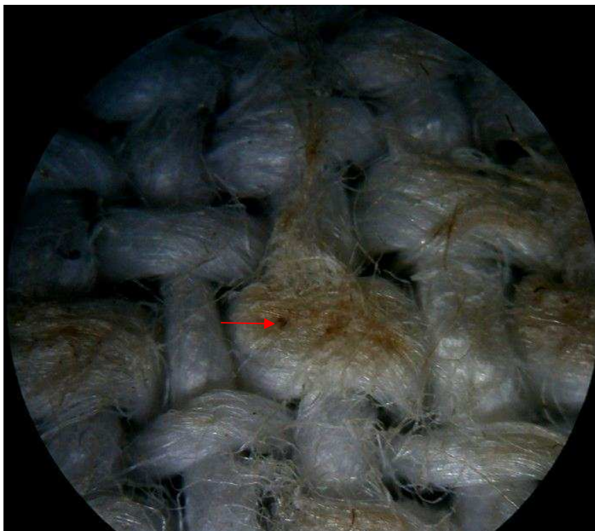
Fig.13: Light Scorch. "Micro hot spot" (arrow).
