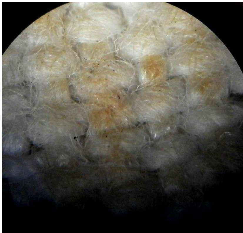
Fig.11: Light Scorch. Typical view. Low magnification.
