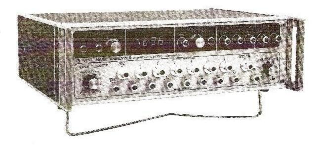
The VP-8 Image Analyzer is the key element in ISI's single channel image enhancement and analysis systems. This versatile instrument operates on a video image input and converts the image data to new display formats for improved visual image interpretation and classification. In addition, the unit allows many quantitative measurements to be taken from the image data.
